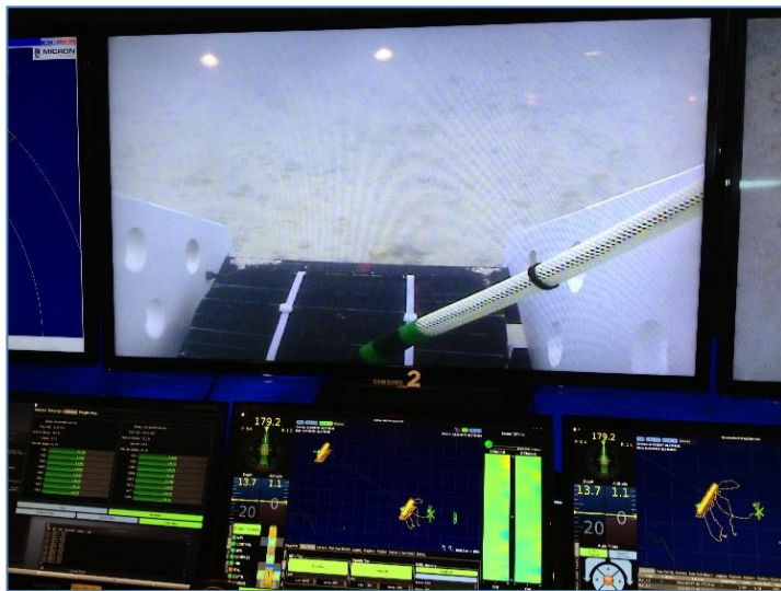
HAUV Dolores control center camera showing Gen-1 EM array being flown over the seafloor
