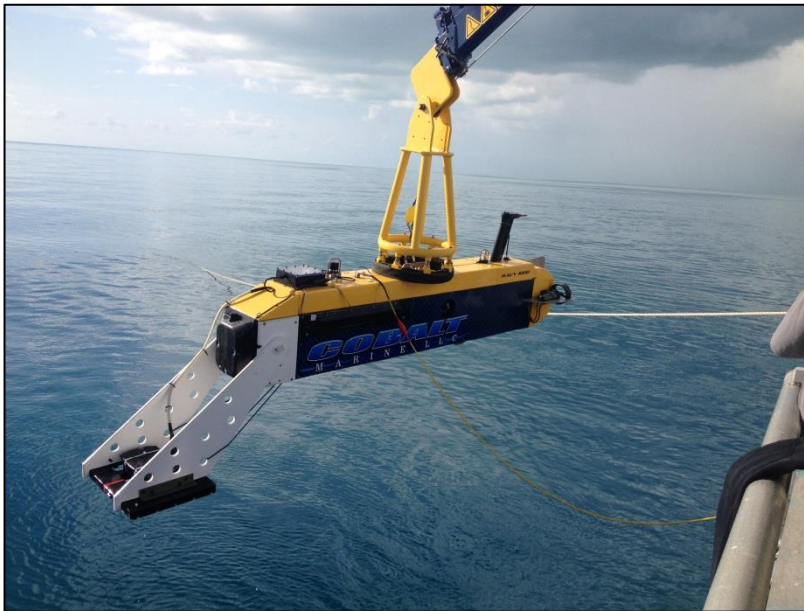
Dolores HAUV being deployed with EM system attached
